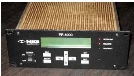
The pressure controllers must be compromised in order to disable the Cascade Protection System's stage exhaust valves. This suggests a link between the Cascade Protection System's main controller, the Siemens S7-417, to the pressure controllers. Since the PR-4000 doesn't come with a built-in PROFIBUS interface, communication is most likely established via a PROFIBUS-to-serial gateway, as shown in the diagram below; a configuration that is used in similar
