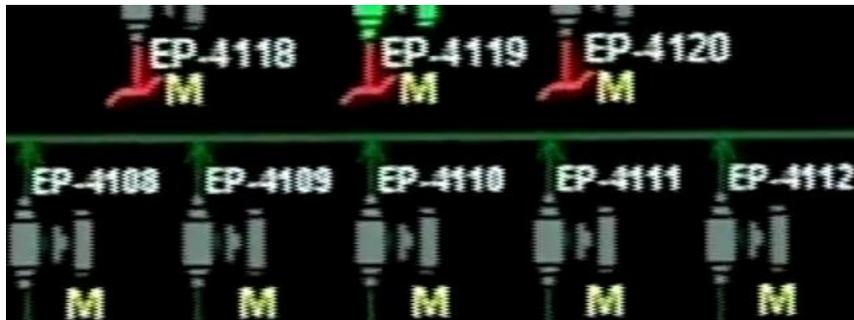
**Figure 8: Very different valves:** While the stage exhaust valves (labeled EP-4108 to 4112 in this partial screenshot from the CPS SCADA display) stay closed during normal operation *and during the attack*, at least one of the feed valves (labeled EP-4118 to EP-4120) must stay open. Pressure controllers at the product and tails take-offs must also be compromised to not signal a low pressure condition.
