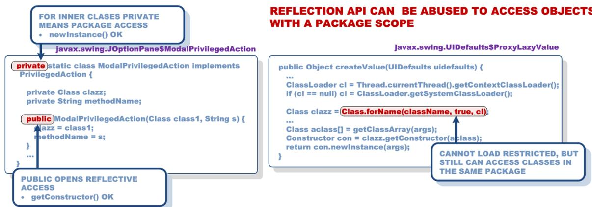
Figure 20. Sample abuse of Reflection API for the creation of package scoped privileged action object.
