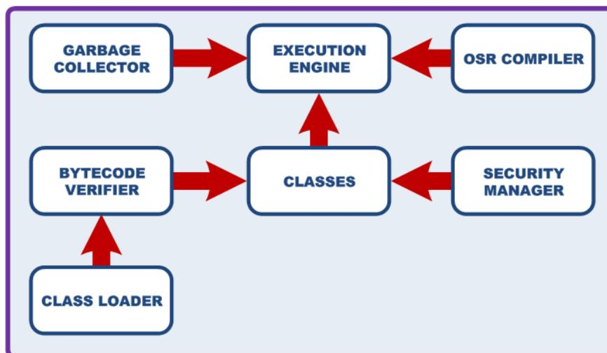
Figure 1. Java Virtual Machine security architecture.
