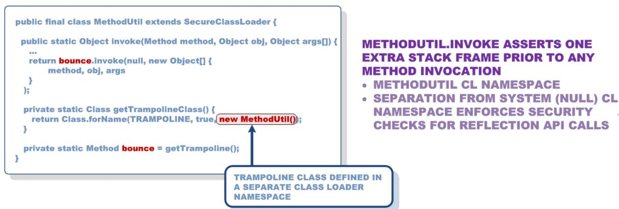
Figure 21. Implementation of `MethodUtil` class as a replacement for reflective `invoke` call.
