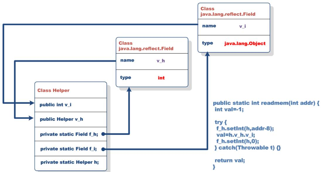
Figure 8. Type confusion condition with the use of Reflection API.
