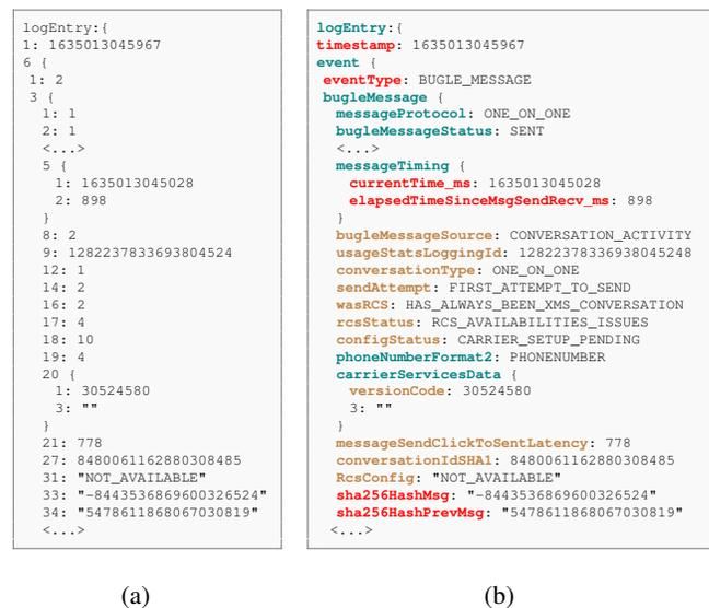
Fig. 7: Example of Google Messages ANDROID\_MESSAGING Clearcut logger log entry: (a) protobuf decoded using Google Protobuf compiler with the `--decode_raw` option, (b) after reverse engineering the schema.
