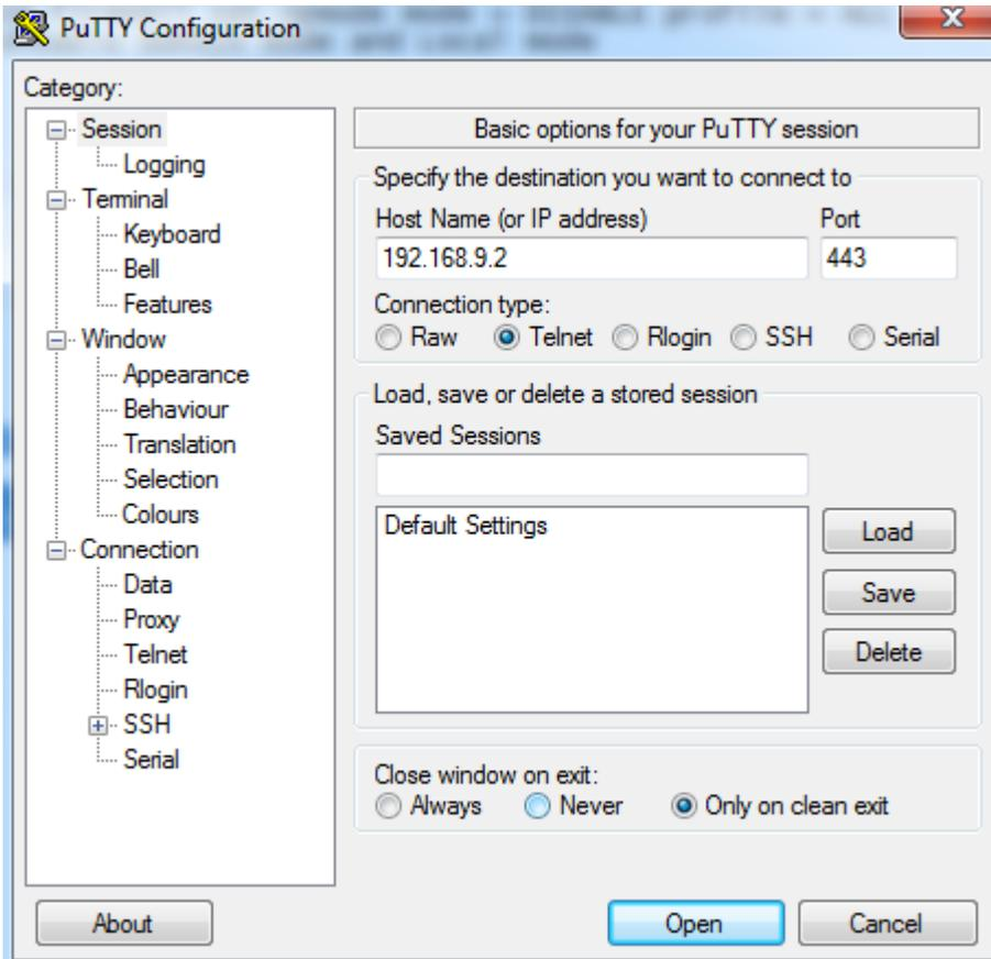
Here the snap shows that we are connecting to 192.168.9.2 via telnet on 443
