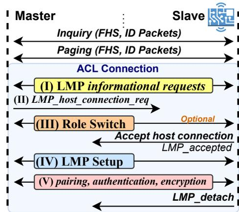
Figure 1: An Illustration of the BT connection procedure. FHS stands for *Frequency Hopping Synchronization*, ID stands for *Identity*, LMP stands for *Link Manager Protocol* and ACL stands for *Asynchronous Connection Less*.
