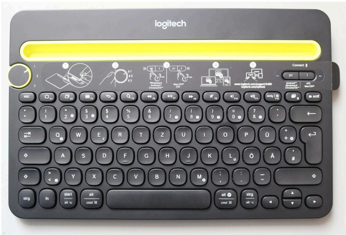
Figure 2: Tested wireless keyboard Logitech K480 with Bluetooth 3.0 technology
