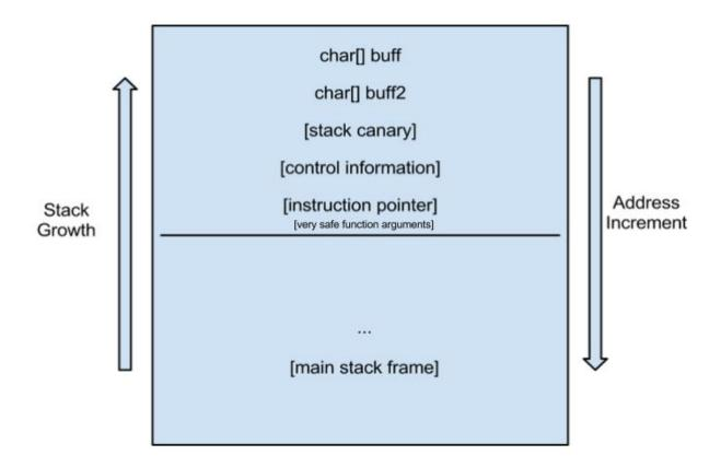
Declaration order often determines the order of the buffers in a stack frame. The buffers are shifted toward the bottom of the stack frame to mitigate exploitation of other local variables, but when there are two buffers one of them must be between the other buffer and the canary. If there is an overflow vulnerability affecting the first buffer, the second buffer can be written to arbitrarily. This is better than allowing complete overflow of local variables, but strings are often easy targets.
