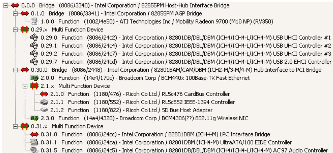
Figure 1: The logical representation of a typical PCI bus
