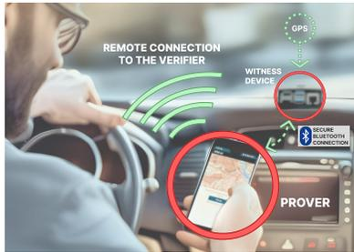
(a) Prototype setup: Android phone (Prover) and Raspberry Pi (Witness) connected via Bluetooth.
