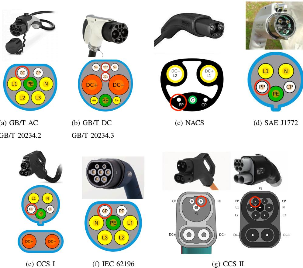
Fig. 2: Charging Gun Standards (Signals from the ports, highlighted in red circles, confirm the proper connection between the EV and the charging pile.)
