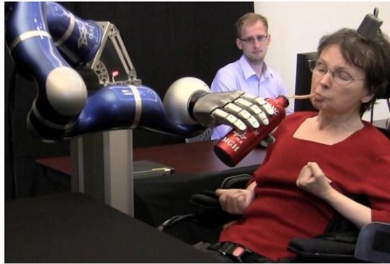
Figure 1.19: A paralyzed person uses a brain-computer interface to control a robotic arm
