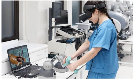
Figure 1.20: VR simulation provides tactile feedback to surgeons
