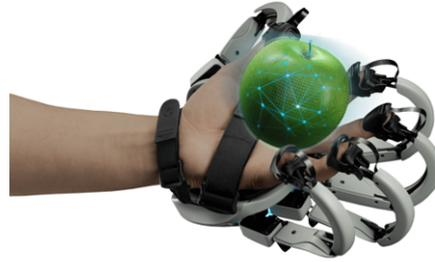
Figure 1.14: Tactile feedback gloves TESLAGLOVE
