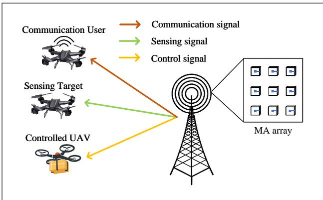
Fig. 4: System architecture of an MA-empowered LAWN.
