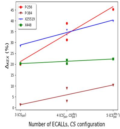
Fig. 6: KEX LURK-T TLS relative overhead over OpenSSL ( $\Delta_{KEX}$ ) in PSK with (EC)DHE mode.
