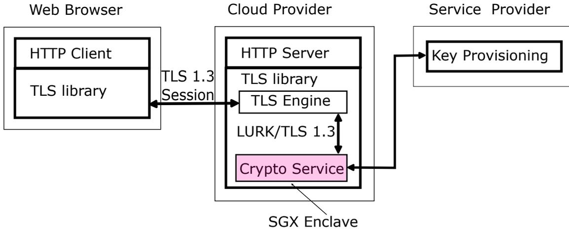
Fig. 1: LURK-T entities: a TLS client  $C$  (a regular web browser), a LURK-T TLS Engine  $E$ , and a LURK-T TLS Crypto Service  $CS$  (both part of a third-party hosting provider), and a key provisioning server (under the content owner’s control).
