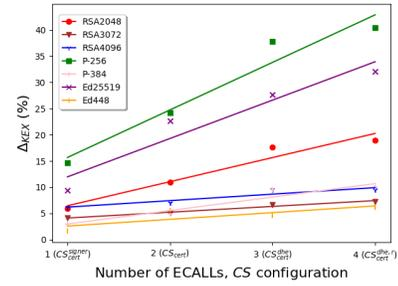
Fig. 5: KEX LURK-T TLS relative overhead over OpenSSL ( $\Delta_{KEX}$ ) in (EC)DHE mode. Measured values are linked using a linear regression.
