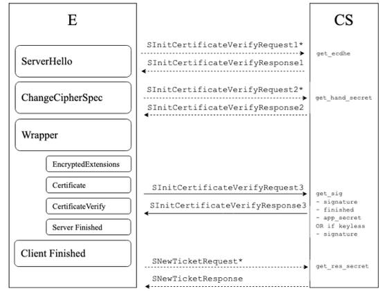
Fig. 4: Messages between  $E$  and  $CS$  for the (EC)DHE mode. \* designates an optional exchange depending on the  $CS$  configuration
