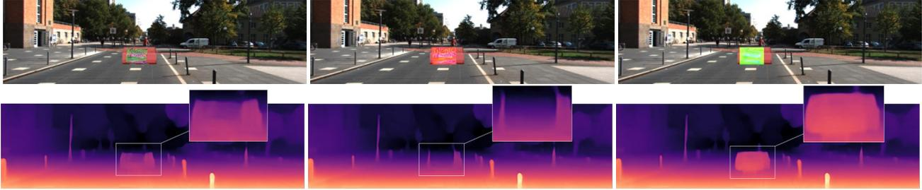
**Figure 7: Visualizations on KITTI dataset. From left to right: SwitchPatch does not affect depth estimation without light projection; SwitchPatch is predicted up to more than 20% farther away than its actual distance when red light is projected; SwitchPatch is predicted up to less than 20% closer than its actual distance when green light is projected.**
