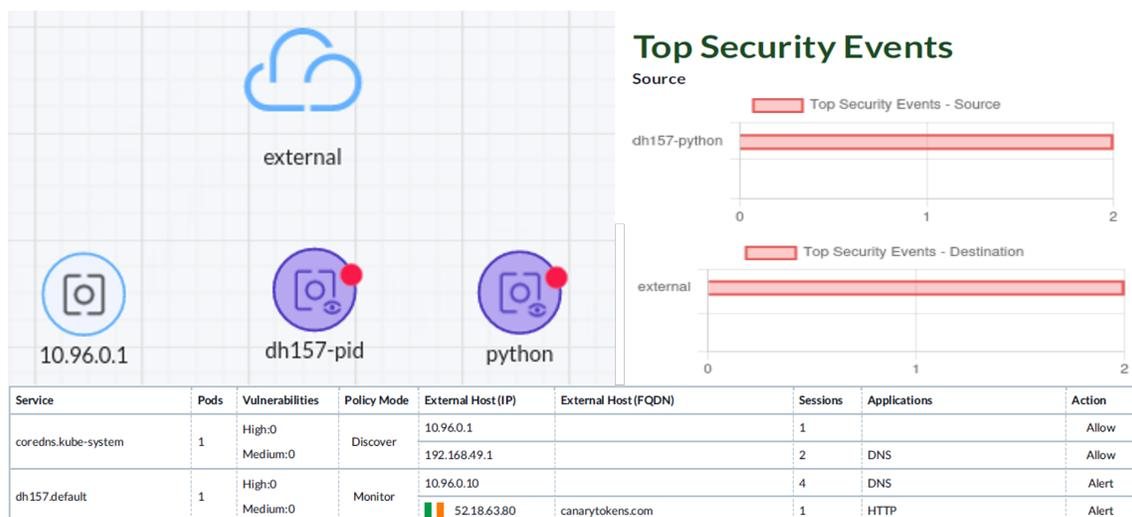
Figure 9: NeuVector Traffic Activity dashboard and Security Alert details (top) and an extract from the summary report (bottom).
