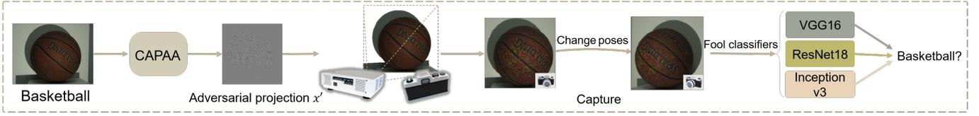
Fig. 3. Overview of the experimental evaluation. First, we sample the object and train PCNet. Then, we use different methods (e.g., CAPAA) to generate the adversarial projections. After that, we project the adversarial patterns onto the object and move the camera to capture the scene in different poses. Finally, the captured images (the object with superimposed adversarial projection) are fed to different classifiers for prediction.
