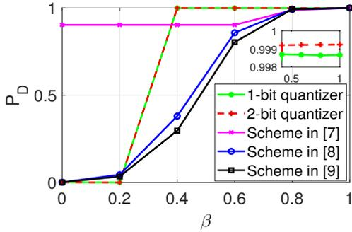
Figure 6:  $P_D$  vs  $\beta$ :  $SNR = 10$  dB,  $P_{FA} = 10^{-3}$
