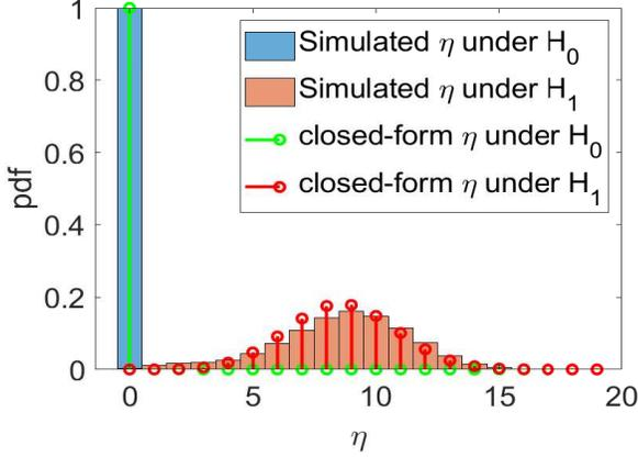
Figure 3: Simulated vs closed-form expression: code rate = 0.01,  $SNR = 10$  dB,  $p_0 \approx 0$  and  $p_1 \approx 0.4539$
