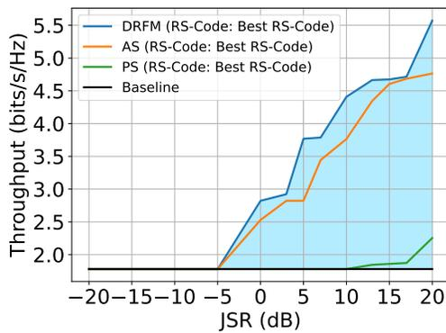
Figure 5: Throughput vs JSR for optimal selected coding rate. Baseline SNR = 10 dB
