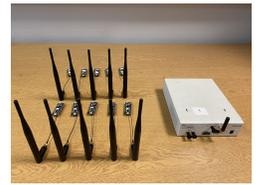
Fig. 5. LoRa transmitters and a USRP receiver.
