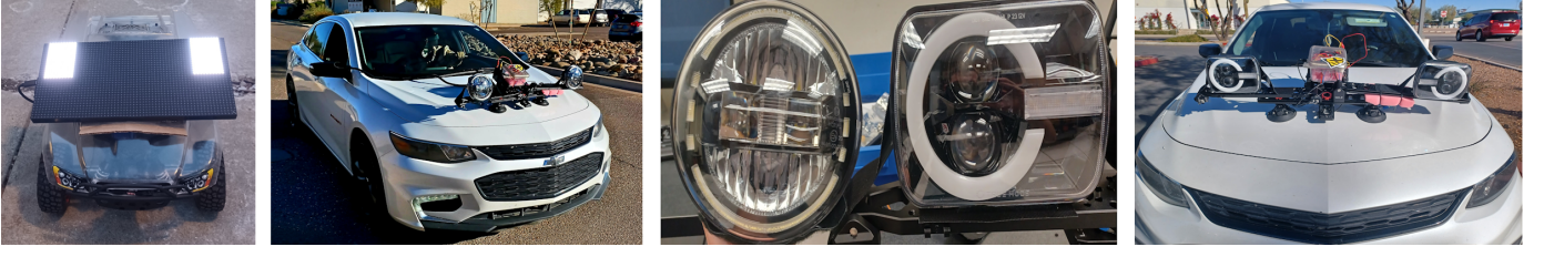
Fig. 4: Implementation of our vehicle setup with RC-car and real-car, showcasing different headlight configurations.
