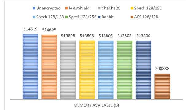
Fig. 15. The figure shows the available RAM under different encryption algorithms.
