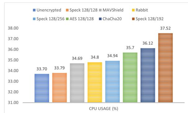
Fig. 17. The figure shows the CPU usage under different encryption algorithms.
