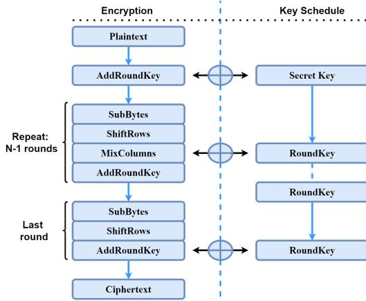
Fig. 6. The figure shows the encryption process of the AES algorithm.
