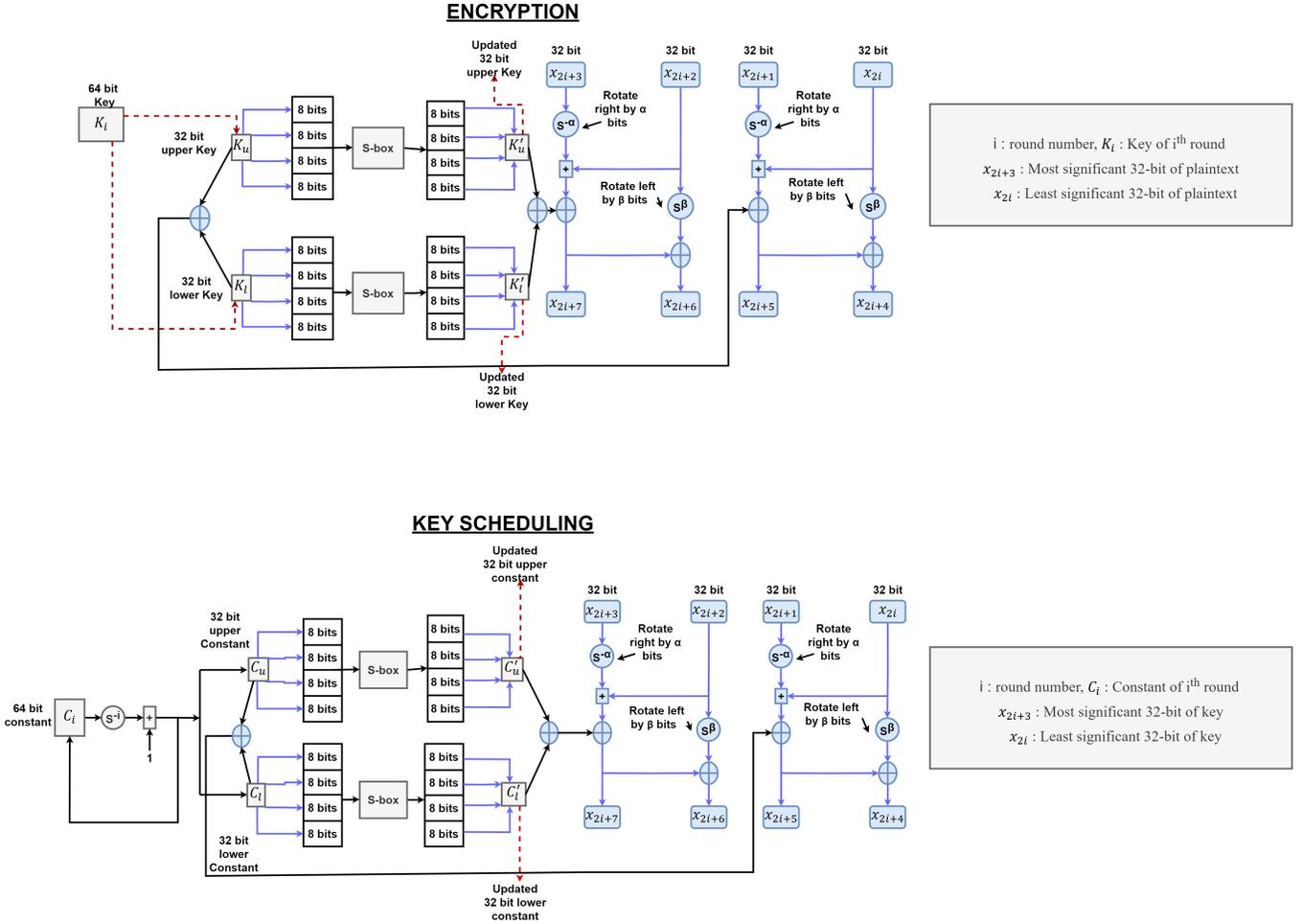
Fig. 8. The figure shows the MAVShield key scheduling and encryption functions.
