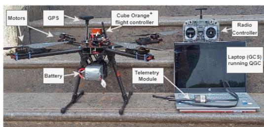
Fig. 11. The figure shows the experimental setup of our drone testbed.
