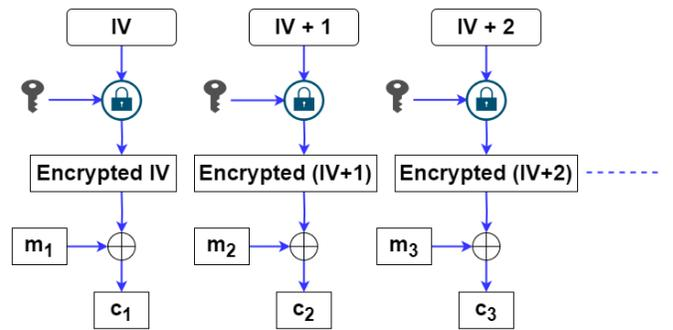
Fig. 5. The figure shows the encryption process in counter mode [29].
