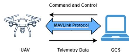
Fig. 1. The figure shows the communication between a UAV and a GCS.
