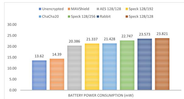
Fig. 16. The figure shows the battery power consumption under different encryption algorithms.
