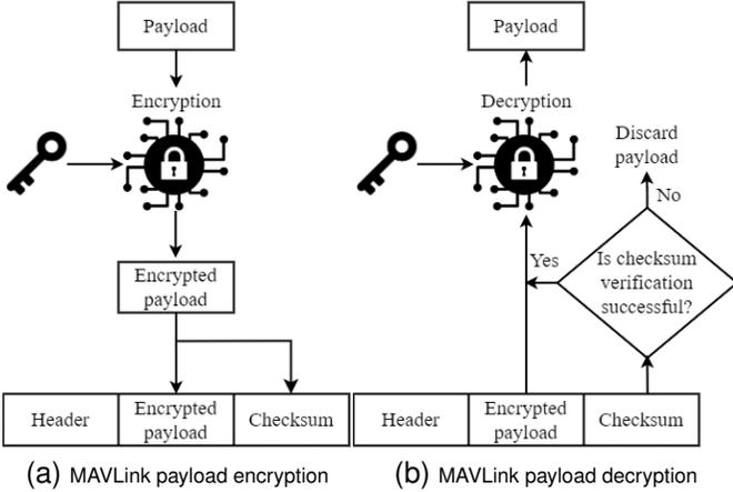
Fig. 4. The figure shows the integration of security algorithms in the MAVLink protocol.
