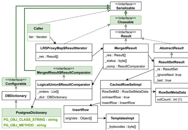
**Figure 6: Payload visualization for dormant *OpenJPA* gadget chain. Modifications are highlighted in green.**
