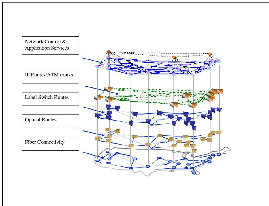
The network control and application services will reside at the uppermost network layer. Layers three and four carry the switching and message routing. Section 4.0 of this document considers the implication of protocols.
