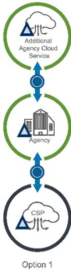
**Option 1:** The first option (left) aligns with traditional mechanisms for connectivity between distributed agency cloud resources, establishing connectivity through the agency campus as described in the Traditional TIC Use Case. Policy enforcement can be performed at the agency campus or the cloud resources. Policy enforcement parity between cloud resources can be simplified by applying protections at the agency campus.
