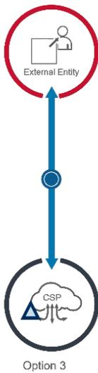
**Option 3:** The **third option** (left) option permits connectivity from external entities directly to cloud resources via protected connections (TLS, etc.). Policy enforcement can only be performed at the CSP, which can potentially facilitate policy enforcement parity and resiliency for cloud resources.
