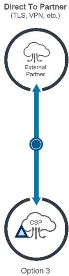
**Option 3:** The **third option** (left) permits direct connectivity between external partners and agency CSP resources via protected connections (TLS, VPN, etc.). Policy enforcement can only be performed at the CSP, which can potentially facilitate policy enforcement parity and resiliency for cloud resources.
