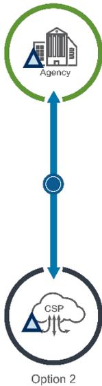
**Option 2:** The **second option** permits connectivity from on-campus agency users directly to cloud resources via protected connections (TLS, VPN, RDA, etc.). Policy enforcement can be performed at the agency campus and the CSP. Policy enforcement parity across multiple campuses can be simplified when policy enforcement is performed at the cloud environment.
