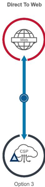
**Option 3:** The **third option** (left) permits connectivity from agency CSP resources directly to web resources. Policy enforcement can be performed at the CSP.
