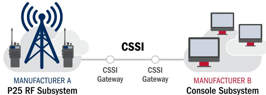
Figure 18 – Console Subsystem Interface
