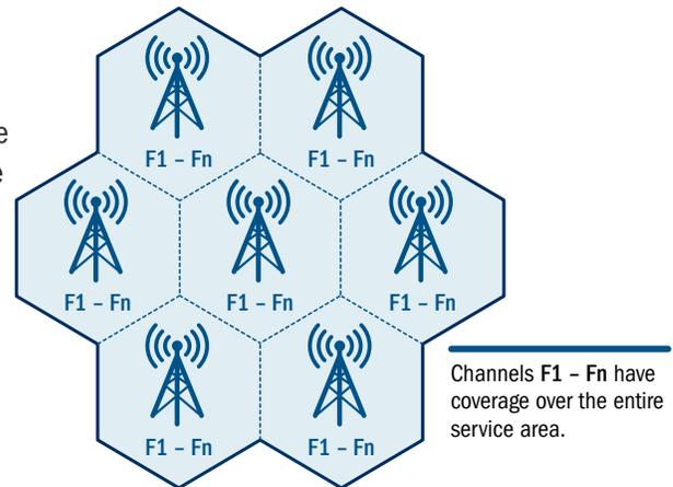
Figure 8 – Simulcast Layout
