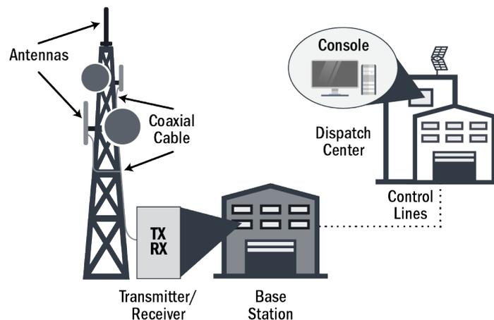
*Figure 17 – Console Subsystem Connected to Base Station*
