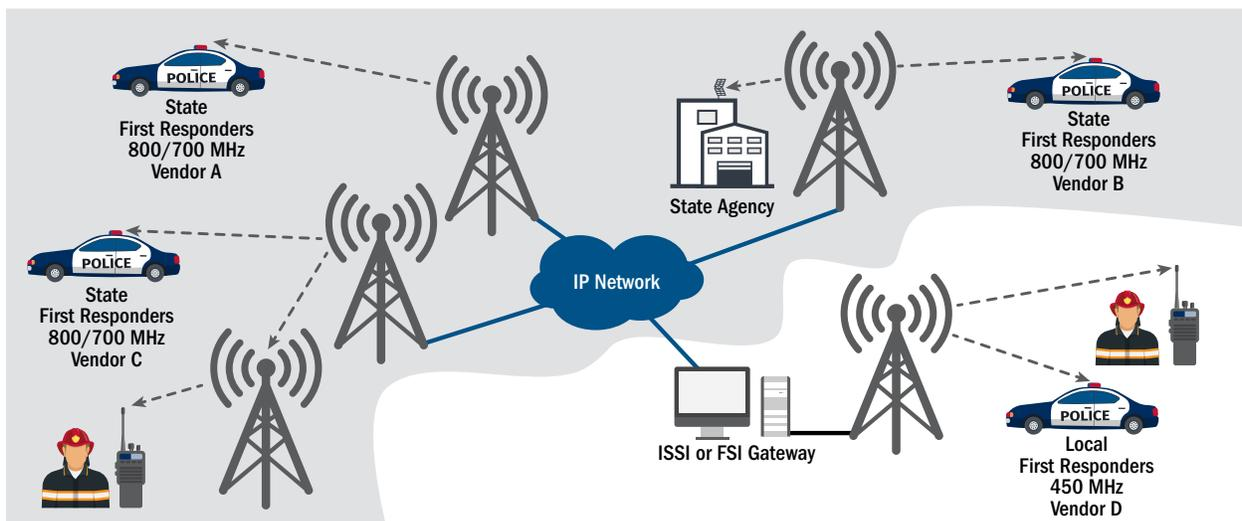
Figure 7 – Wide Area P25 Network with IP Backhaul
