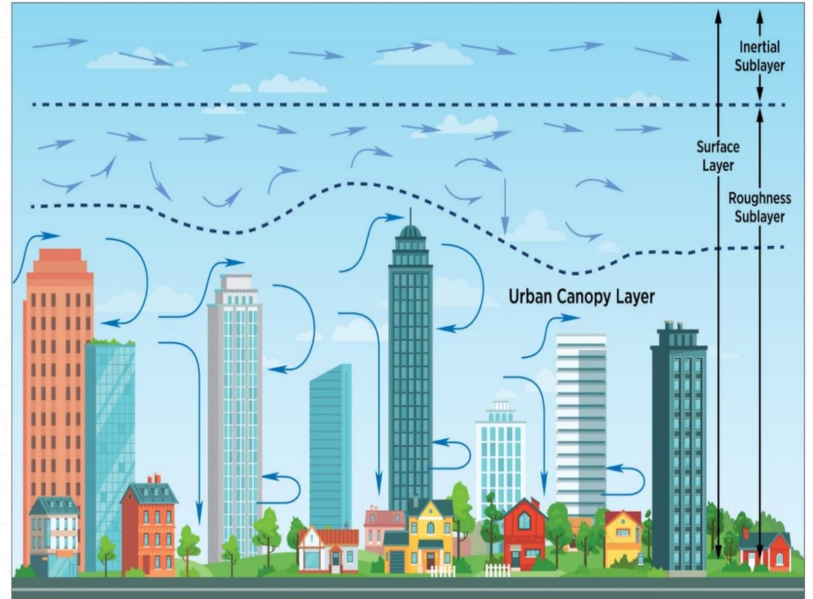
Schematic of flow through and over an urban area
