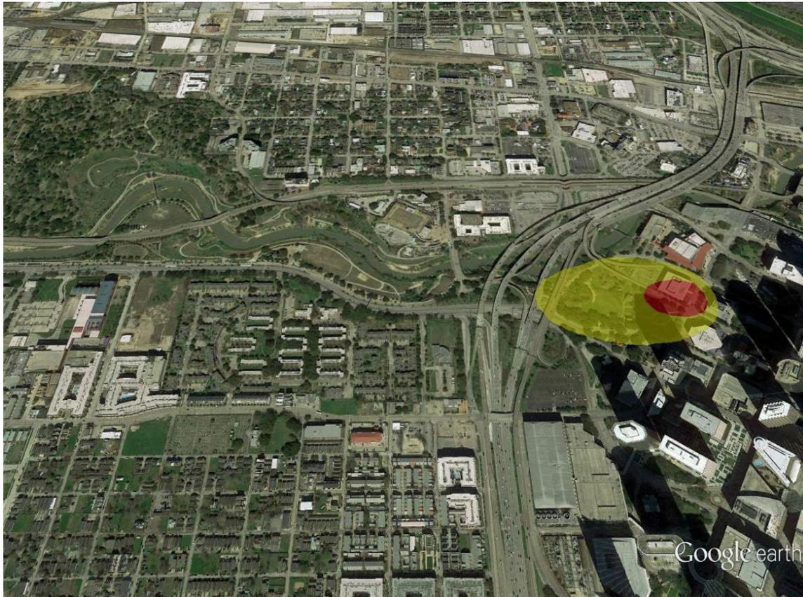
Modeling 50-ton ammonia release as atmospheric gas cloud
