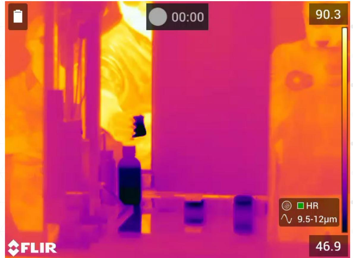
An infrared detector is used to visualize the resulting plume after liquid ammonia is poured into a beaker containing 4% ammonia in water (left) and poured onto a concrete coupon (right)
