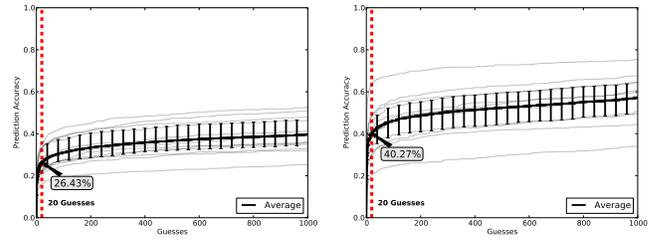
**Figure 15:** Prediction accuracy for bigram HMM over multiple guesses for patterns (*left*) and PINs (*right*), and the 20 guess threshold is indicated with a dashed line. The shaded trend lines are individual users. Note that PINs outperform pattern prediction, likely due to the limited number of transitions and shorter sequences.
