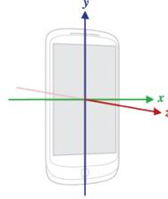
**Figure 2:** Accelerometer Axis of Measurement (Source [10])
