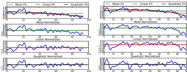
**Figure 4:** Visual example of normalization: In the top plot, the raw accelerometer data is presented with the appropriate mean, linear, and quadratic fits, and following plots show the affect on the raw accelerometer data when normalized to those fits, respectively.
