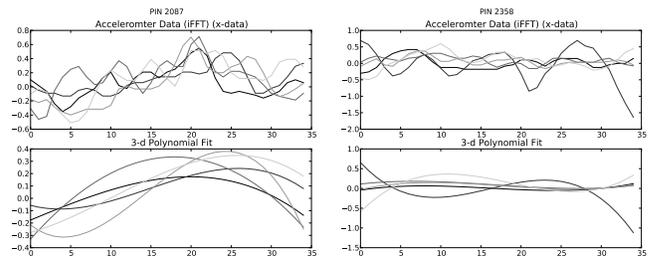
**Figure 5:** An example of polynomial fit features for PIN 2087 (left) and PIN 2358 (right). The top plot shows iFFT-ACC of the accelerometer data (just acceleration in the  $x$  dimension), and the bottom plot shows the 3-d polynomial fit (iFFT-Poly).
