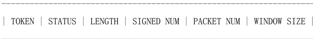
The field TOKEN is one byte, which shows packet type. In this article, it is 0x12, which shows the request of ConnectionPreLogin to get some values, such as the version of SQL Server. When SQL Server receives these kinds of package, it will pass the package to function in SSlibnet.dll. In my SQL Server with no SP, the function is list as following:
