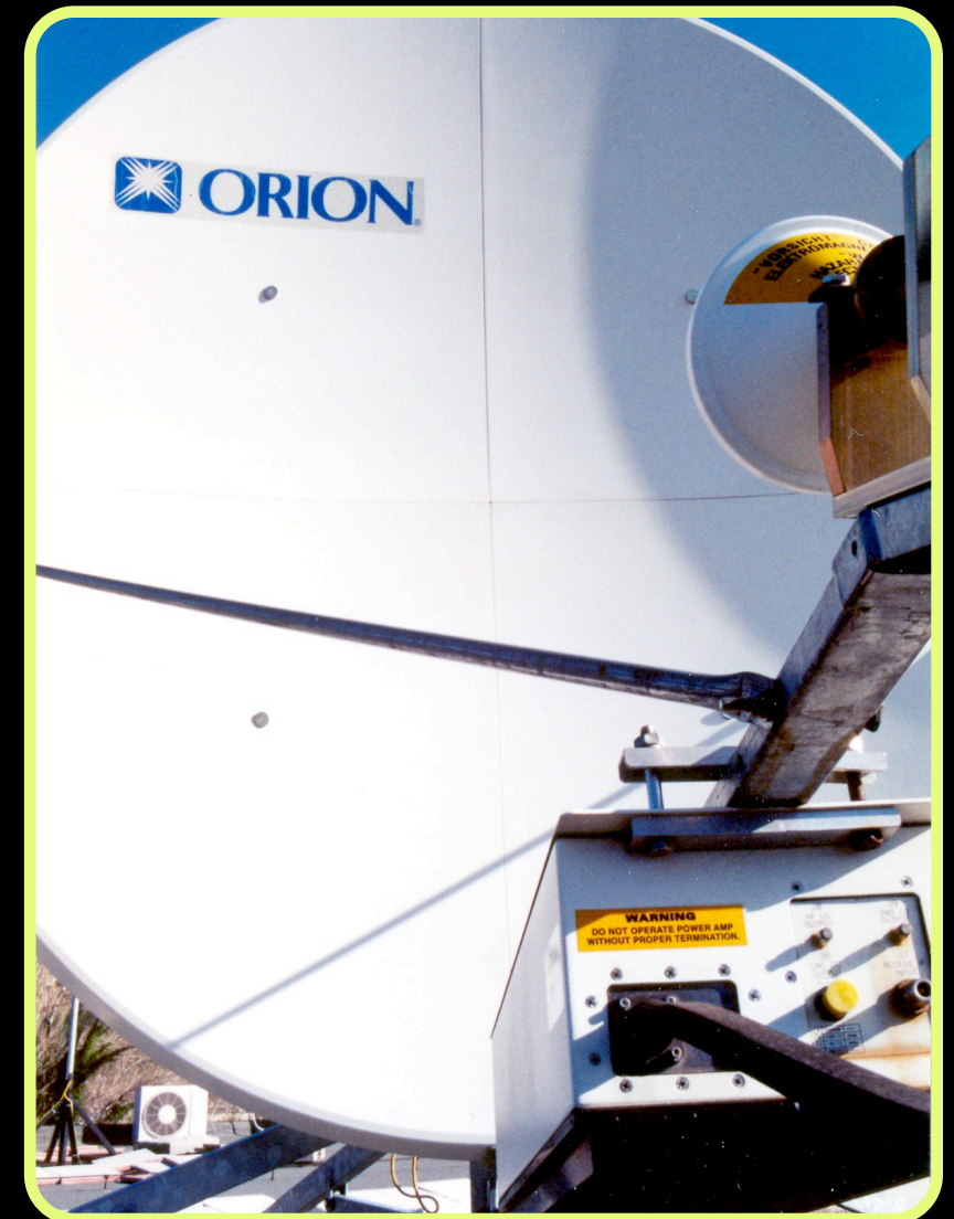
A 2.5m parabolic dish antenna for bidirectional high-speed satellite Internet. source: http://en.wikipedia.org/wiki/VSAT
