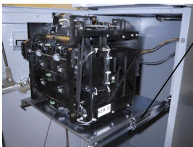
*Mechanism in operating position. If unit is slide-mounted, release locking tab and slide dispenser into cabinet.*
