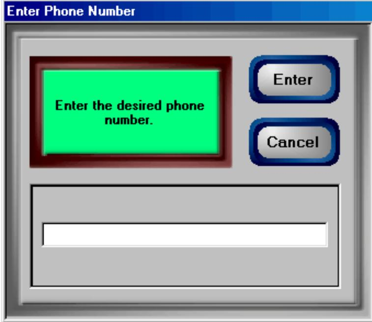
Use this function to test the Cash Dispenser's modem. Enter a known good telephone number, which the modem will dial to verify its ability to access the telephone line and perform a dialing operation.
