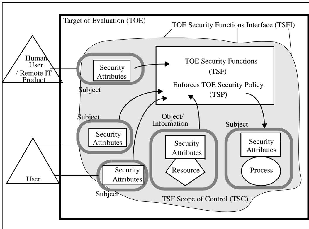
Figure 1.1 - Security functional requirements paradigm (Monolithic TOE)
