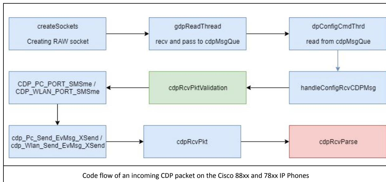
The majority of the above flow simply sets up a RAW socket to capture the CDP packets, while the validation of the packet occurs in the function *cdpRcvPktValidation*:
