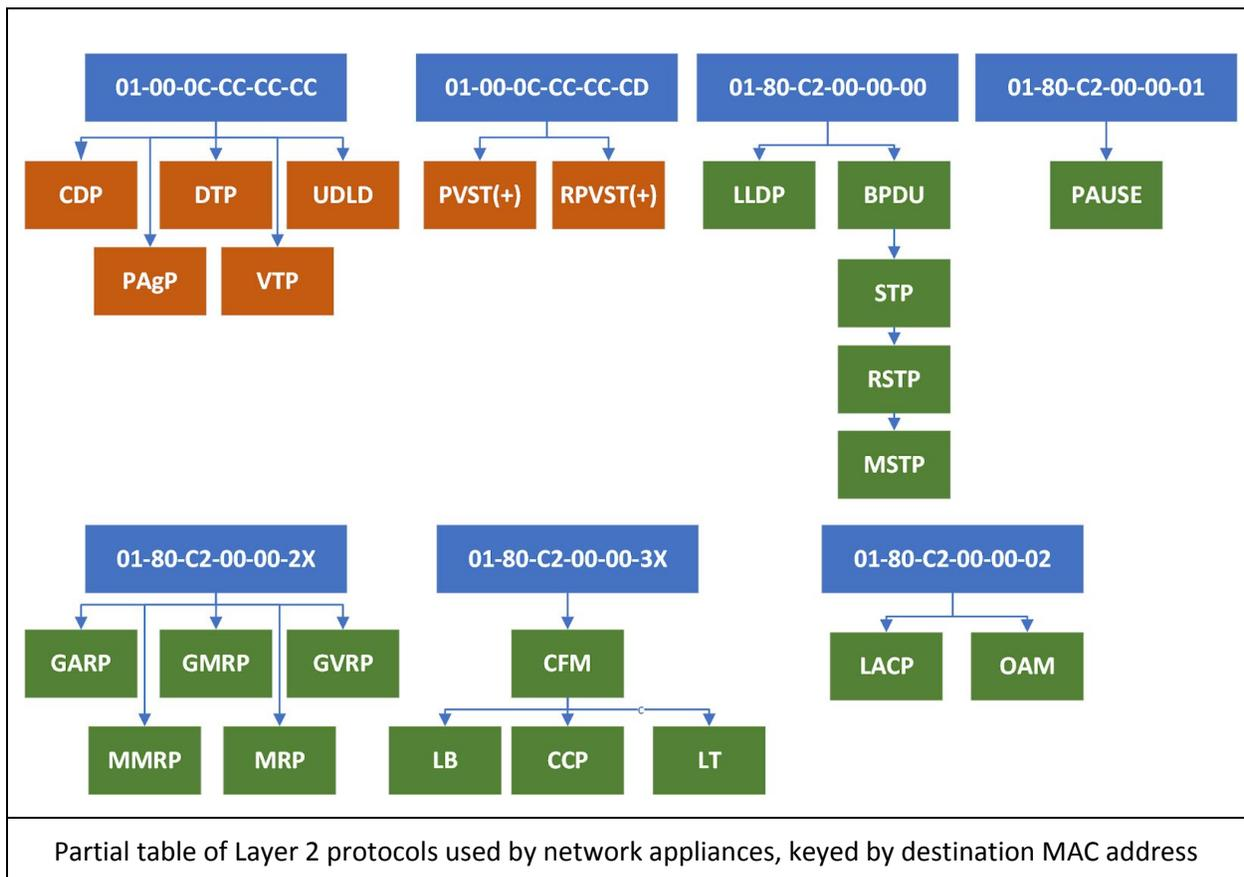
While examining a Cisco Nexus switch, for example, we found that many of these Layer 2 protocols are eventually handled by software. Nexus switches are based on the NX-OS operating system which is based on Wind River Linux.
