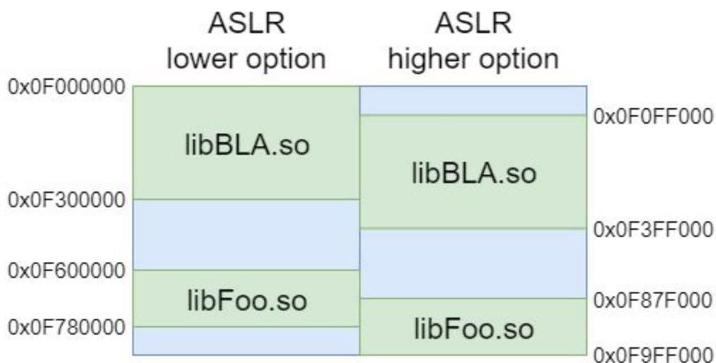
For example, In the illustration above, address 0x0F100000 is a valid executable address for all possible ASLR shifts. Using the above limitation of ASLR in the CDP daemon, an attacker can develop an exploit that will use a ROP chain that will handle concurrent options for the ASLR shift, and can thus dramatically limit the effect of the ASLR mitigation.
