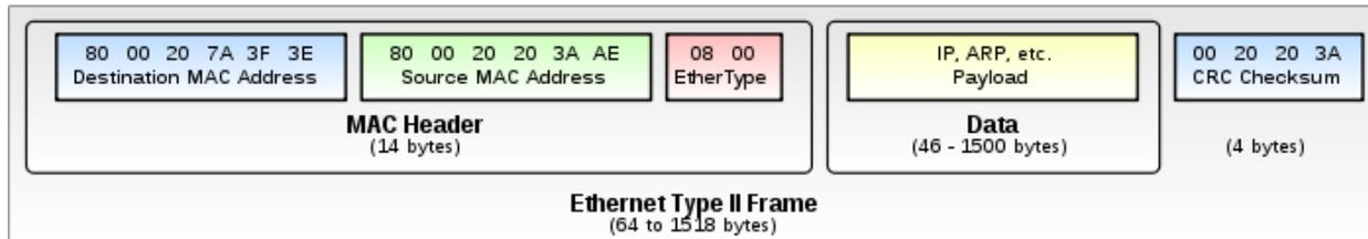
The 16-bit EtherType field in the Ethernet header can actually also function as the Length field of the Ethernet frame:
